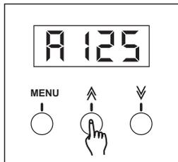
2. Each tap of the Up or Down arrow buttons will change the DMX address value once. Pressing and holding down either the UP or Down arrow buttons will increase or decrease the DMX address setting quickly. Once the DMX address channel is achieved, release the UP or Down arrow button. The new address setting will automatically be stored into memory..
