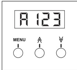
1. Press the "MENU" button until the letter "A" appears in the left hand side of the display. The display will show the "A" followed by the current address setting. For example, if the last set DMX channel was 123, your display should look like our picture to the left.
