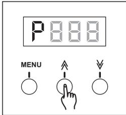
4. Tap the Up or Down arrow buttons to enter a dim preset value within the range of 00-100. Each tap will increase or decrease the value once. Pressing and holding the UP or DOWN arrow buttons will change the value quickly.
