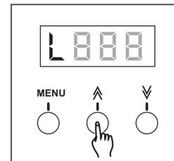
4. Tap the Up or Down button to increase or decrease the value within the range of 10-100. Each tap will increase or decrease the value once. Pressing and holding the UP or Down arrow button will increase or decrease the value quickly.
